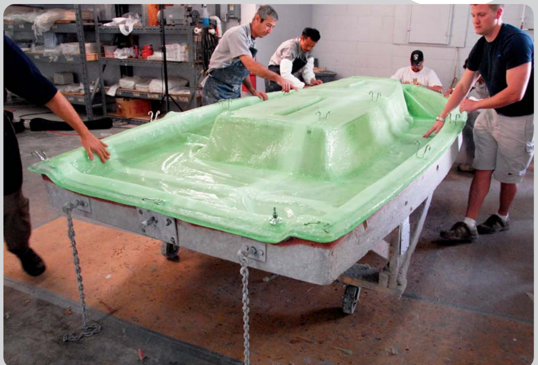
Silicone bag being positioned over composite moulding
